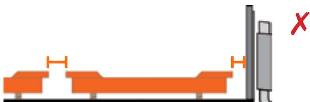
Unblocked load if total gaps are larger than 200mm
