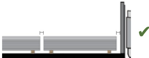
Max 200mm total gap to blocking surface for Blocked loads
