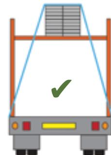
Ensure lashings are attached to the truck deck
