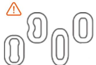
Chains with elongated, worn or bent links must not be used for restraint
