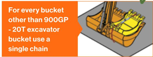
Restrain each individual nested bucket with an 8mm belly chain tensioned to min. 750kg.f to prevent movement,
