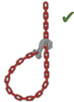
Permitted on up to 3.5t compaction equipment.
