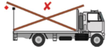
Do not position scaffold planks on an angle
