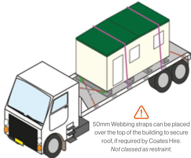
50mm Webbing straps can be placed over the top of the building to secure roof, if required by Coates Hire. Not classed as restraint.
