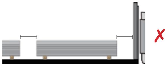
Unblocked load if total gaps are larger than 200mm
