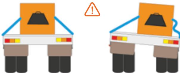
Small building movements are expected during transit resulting in chain slack, cable ties will prevent chain hooks becoming detached from the chain
