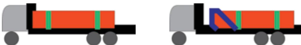
**Example - Blocked with cross-over chains and tie-down chains**
