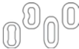
Chains with elongated, worn or bent links must not be used for restraint
