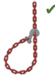
Single loop chains permitted on some smaller machines where specified e.g. Scissor lifts to 7.5t.
