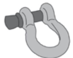
Bow shackles rated to 4 x lashing capacity of chain. Maximum of 2 chains.
